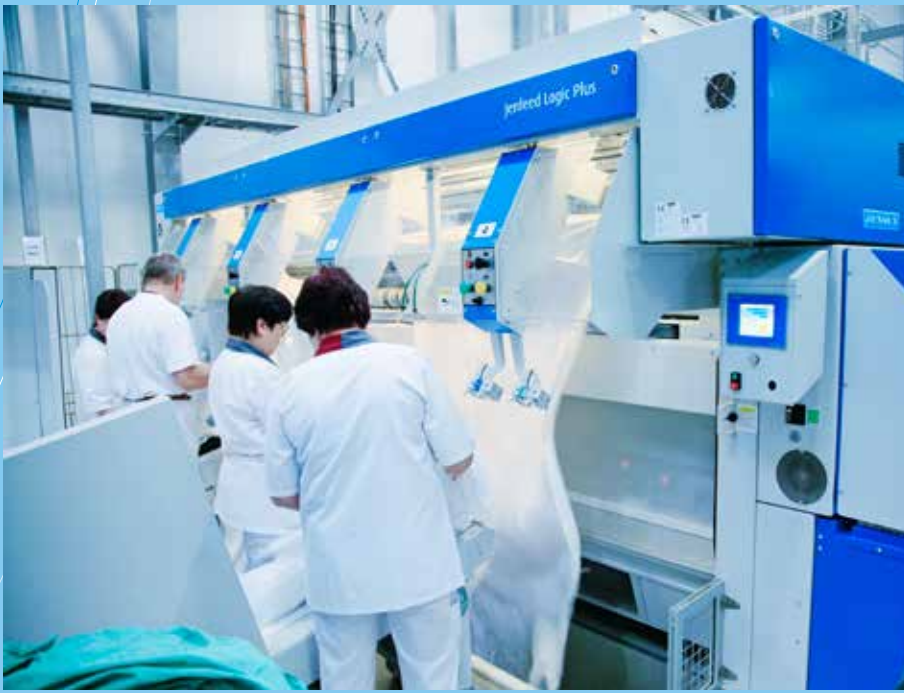
Example of typical installation comprising delivery of linen on conveyors between operators
