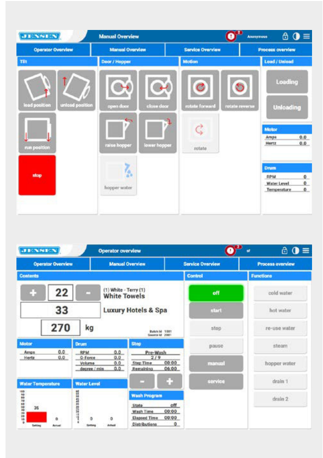
The JWE 270/600 runs on the JOS operating system, for easy and full control of all aspects of machine performance.
