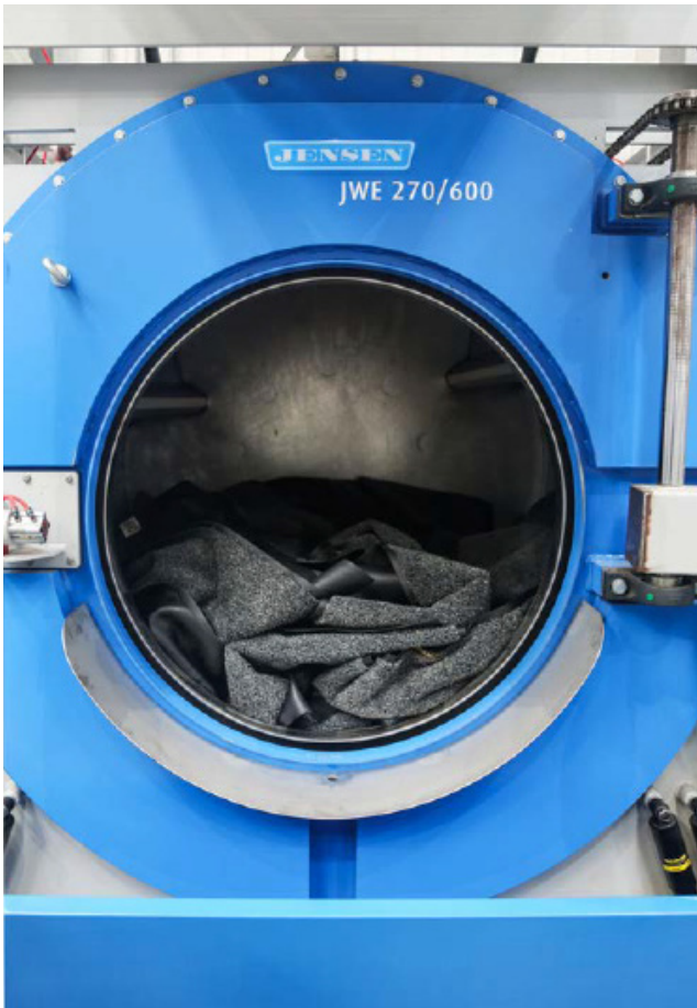
The JWE 270/600 is designed for big loads and can handle mats as well as garments and delicate linen.
